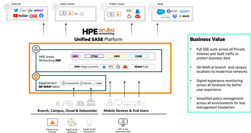
**Figure 3.** HPE Aruba Networking unified SASE platform
