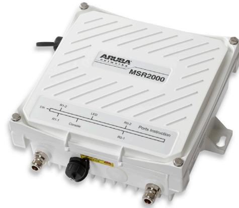
Aruba's MobileMatrix™, another key MeshOS Layer 3 technology, allows Wi-Fi clients to move between wireless mesh routers in less than 50 milliseconds, maintaining a seamless connection for latency-sensitive applications, such as video and voice.
