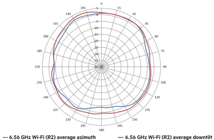
Figure 3. 6.56 GHz Wi-Fi antenna patterns (horizontal)
