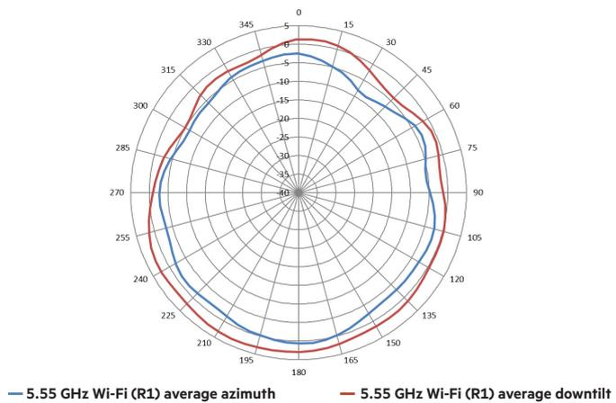
Figure 2. 5.55 GHz Wi-Fi antenna patterns (horizontal)
