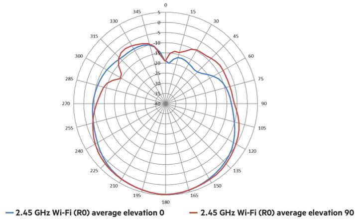
**Figure 4.** 2.45 GHz Wi-Fi antennas patterns (vertical)
