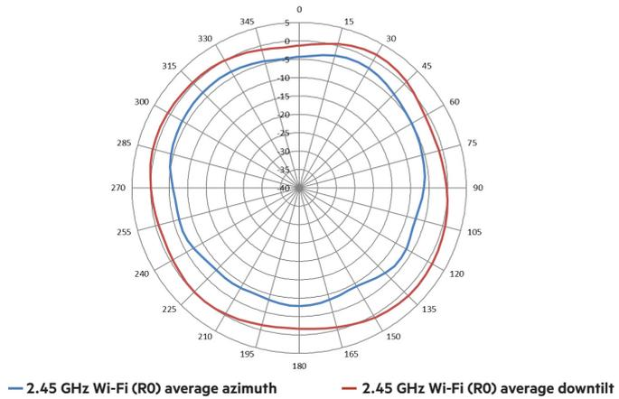
Figure 1. 2.45 GHz Wi-Fi antenna patterns (horizontal)
