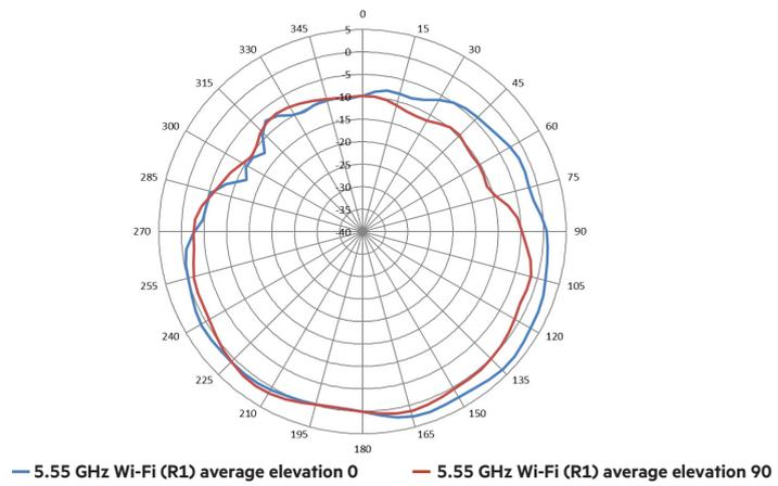
**Figure 5.** 5.55 GHz Wi-Fi antenna patterns (vertical)
