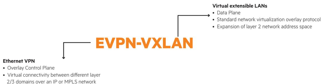
**Figure 3.** EVPN/VXLAN standards-based overlay fabric
