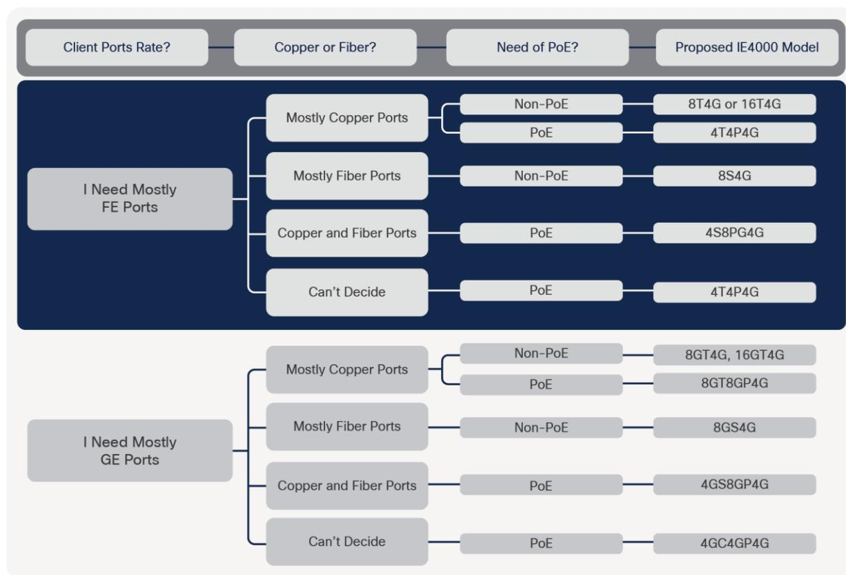
**Figure 2.** Cisco IE 4000 model selection guide
