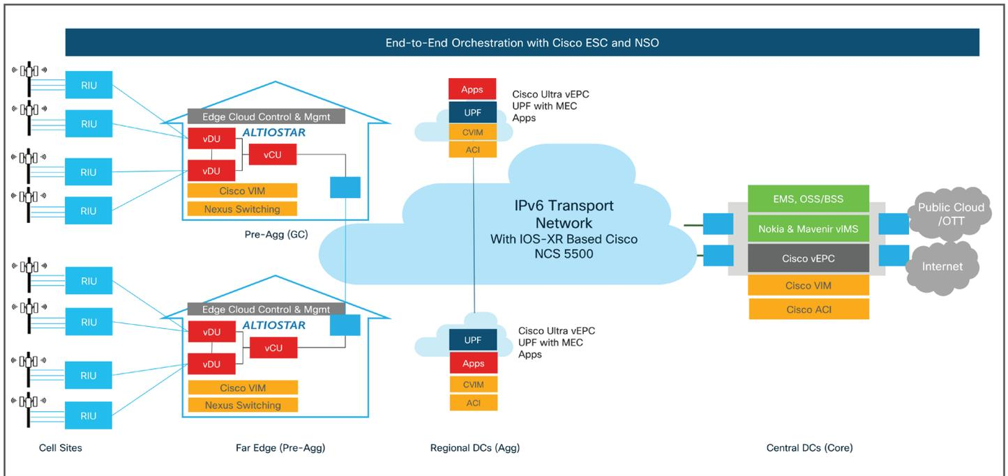
The architecture enables a lean cell site for RMN comprising the antenna and remote radio head. It supports coordinated radio processing to increase spectral efficiency, facilitates scale out, and exposes open APIs that enable multiple vendors to participate and contribute.
