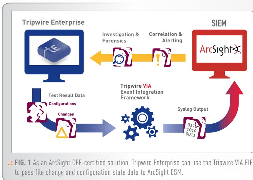
FIG. 1 As an ArcSight CEF-certified solution, Tripwire Enterprise can use the Tripwire VIA EIF to pass file change and configuration state data to ArcSight ESM.
