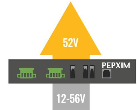
Voltage regulation and boost, monitor battery health on the cloud, low power disconnect.
