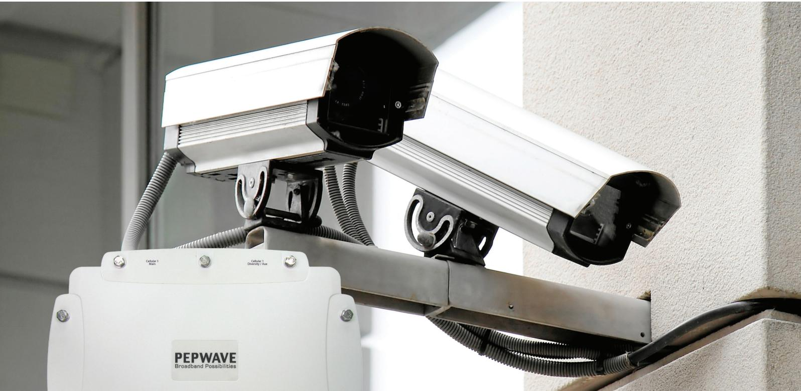
The HD2 IP67 offers dual embedded cellular modems and PoE support, all encased in a shock and vibration certified, waterproof enclosure that's more than a match for almost any environment.
