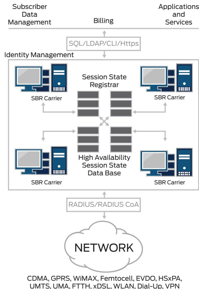
Figure 3: SBR Carrier with its SSR module deployed in a cluster configuration
