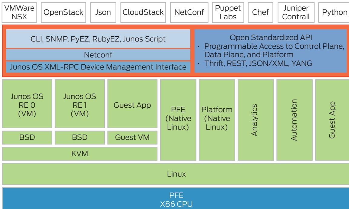
Figure 2: Juniper Virtualized Open Network Operating System Framework
