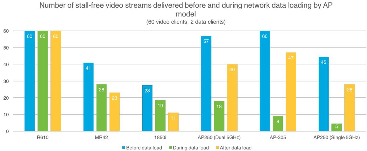
Figure 9 - Test 2 results for number of video supported video clients with and without load
