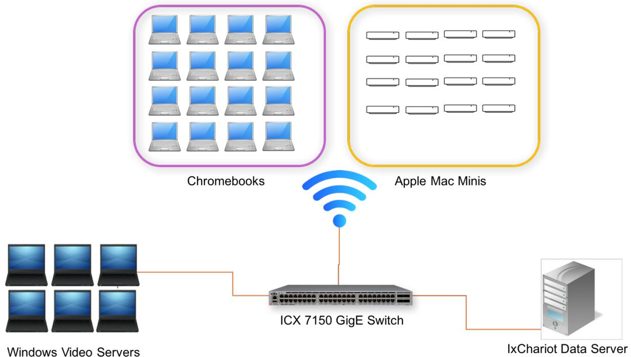
*Figure 2 - Testbed Network Topology*
