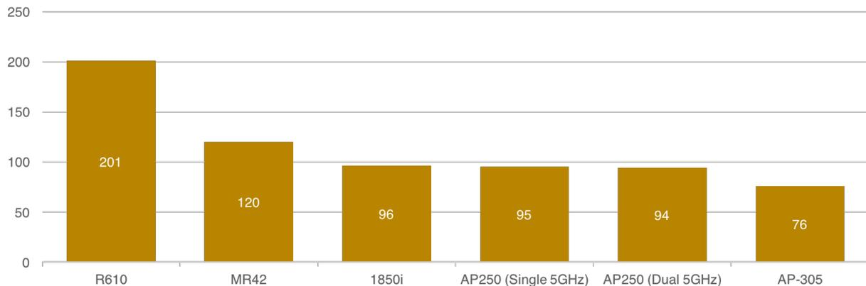
Figure 7 - Test 1 results for aggregate data throughput
