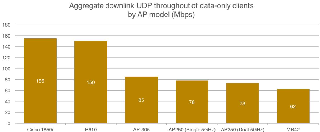
Figure 10 - Test 2 results for aggregate data throughput
