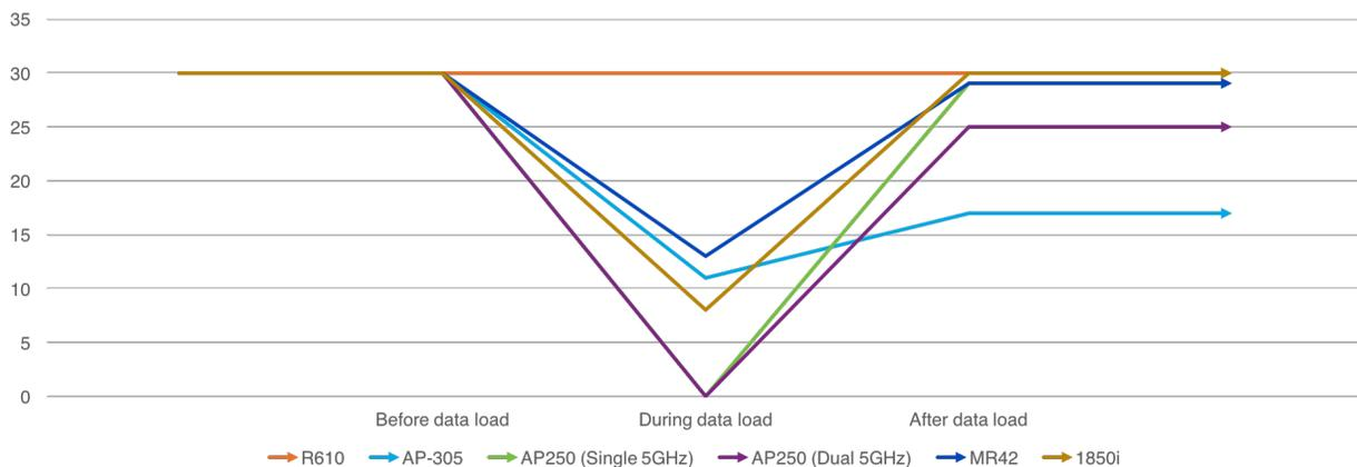
Figure 6 - Test 1 results before, during, and after network data load
