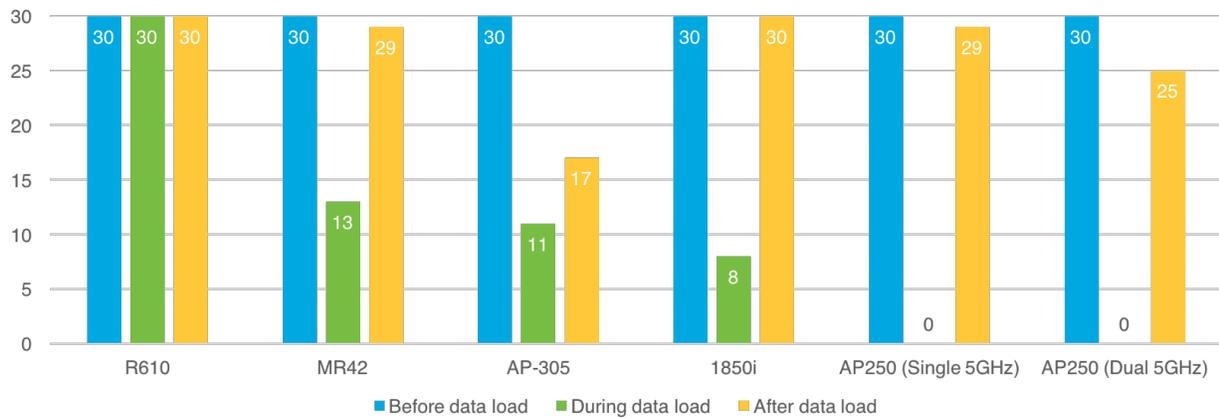
Figure 5 - Test 1 results before, during, and after network data load
