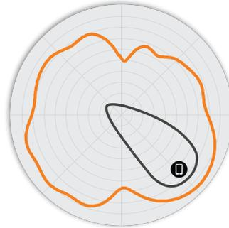
Figure 5. R650 5GHz Elevation Antenna Patterns
