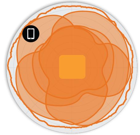
Figure 2. R560 2.4GHz Azimuth Antenna Pattern
