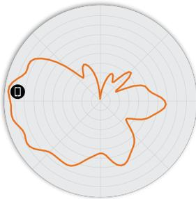
Figure 3. R560 5GHz Azimuth Antenna Pattern
