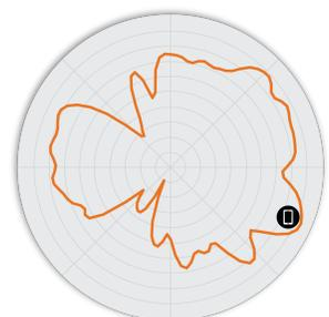
Figure 5. R560 2.4GHz Elevation Antenna Pattern
