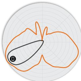
Figure 7. R560 6GHz Elevation Antenna Pattern
