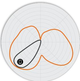
Figure 6. R560 5GHz Elevation Antenna Pattern
