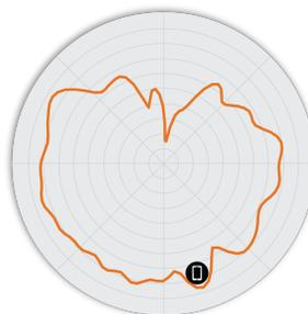
Figure 4. R560 6GHz Azimuth Antenna Pattern
