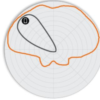
Figure 5. R610 5GHz Elevation Antenna Patterns
