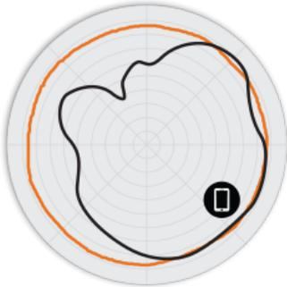
Figure 3. R610 5GHz Azimuth Antenna Patterns
