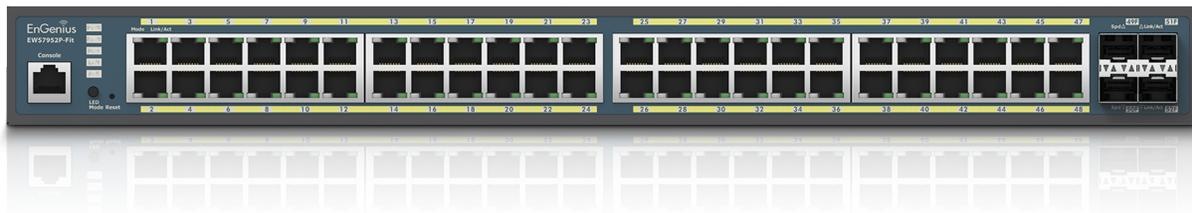
The EnGenius Fit Managed Switch EWS7952P-FIT is a 48-port Gigabit PoE+ Layer 2 plus switch with a 410W PoE budget and 4 SFP uplink ports.
