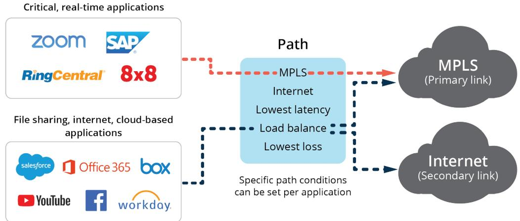
second policy that directs storage replication traffic across the link (or bonded tunnel) delivering the highest throughput capacity.
