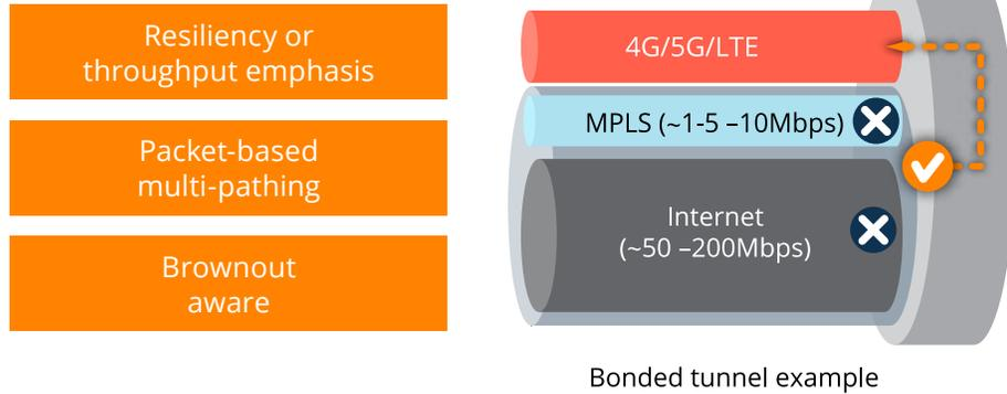
overlay connection. As an example, bonded tunnels can be configured with two MPLS connections to create a primary bonded tunnel. One MPLS connection might be serviced by AT&T and the other by Verizon.
