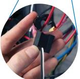
Clamp-on voltage sensors attach to existing branch circuits and monitor voltage while powering the electronics module.
