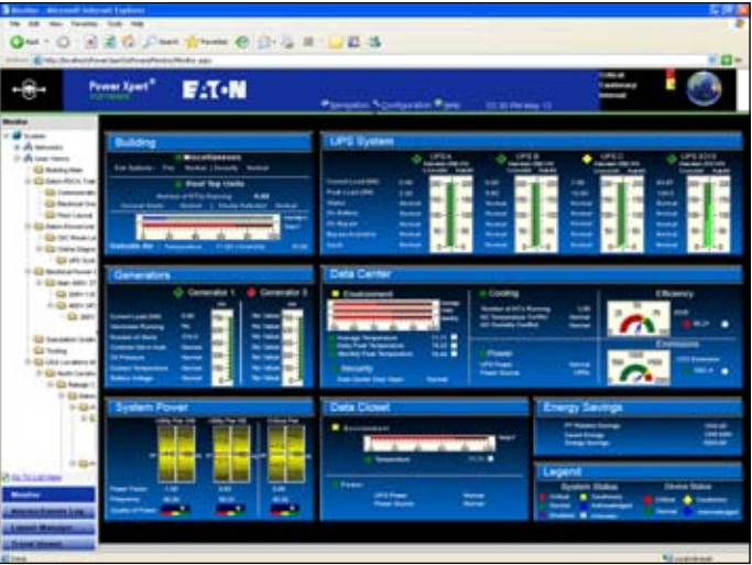
Power Xpert software was designed to seamlessly handle Eaton’s communicating equipment in a graphical manner without additional serial interfaces, protocols or customization.
