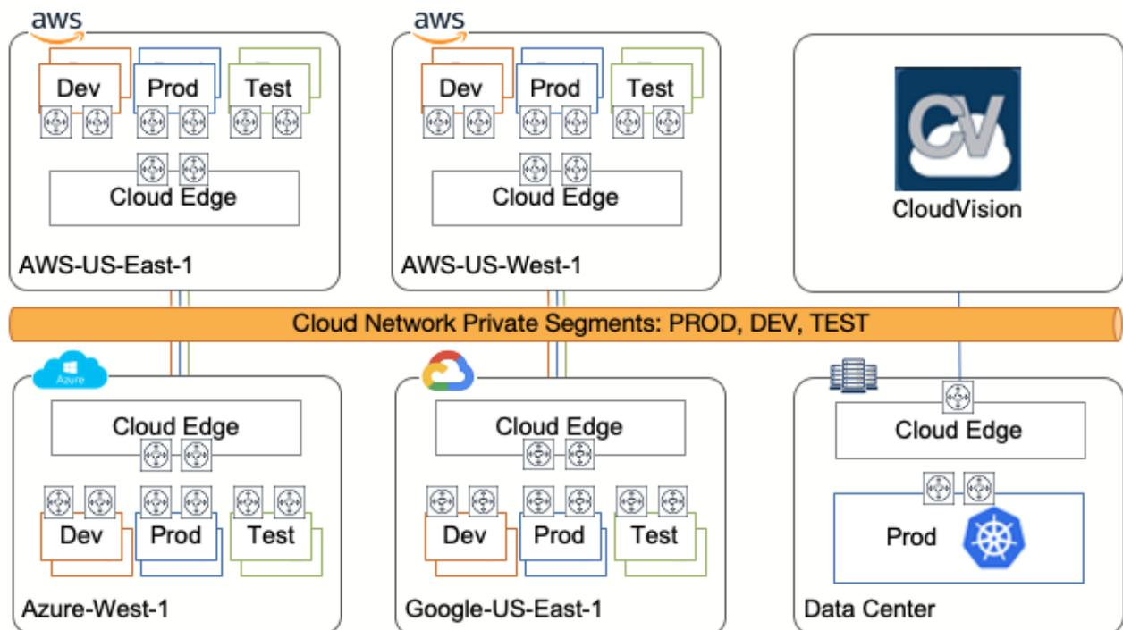
A foundational network construct to enabling our vision of highly reliable cloud operations and concurrent isolation for sensitive workloads is the delivery of Cloud Networking Private Segments (CNPS) over a universal leaf-and-spine topology (figure 3.). The CNPS is a standards-based multi cloud network segmentation method that provides several key capabilities in the increasingly complex enterprise environment for segmentation within and across public and private clouds using a BGP based EVPN.
