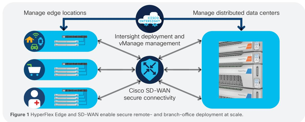
Figure 1 HyperFlex Edge and SD-WAN enable secure remote- and branch-office deployment at scale.
